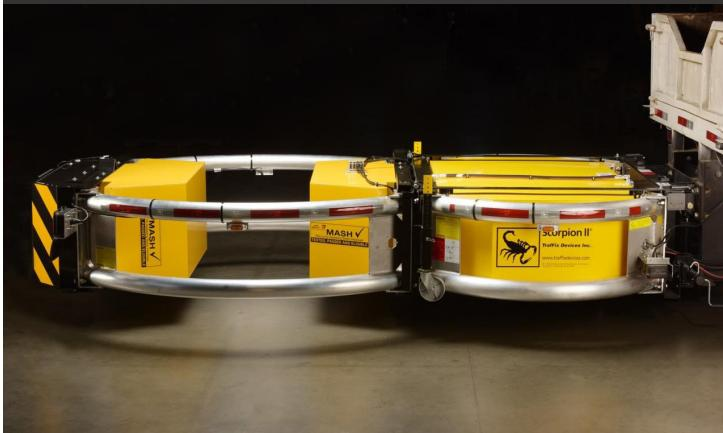
The Scorpion II TMA (Truck Mounted Attenuator) represents a highly advanced, safety-focused crash attenuation system. Its design comprises strut and cartridge sections on a support frame, featuring an open cartridge design to minimize wind resistance and boost fuel efficiency. This system performs optimally both at highway speeds and during stationary work site deployments.
